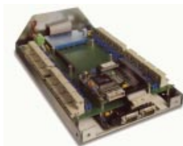
PC 104 single-board for small, energy-minimized systems
