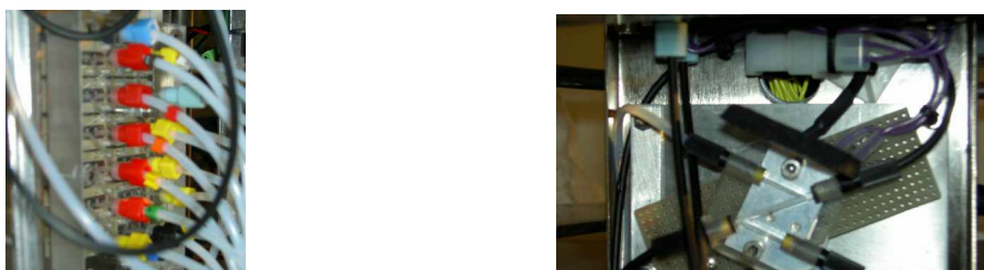
Figure 5. (Left): \mu LFA hydraulic manifold (Right): Miniaturized colorimetric flow-cell with fiber optics couplings.
