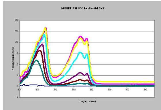
**Fig.5 Typical UV spectra of tri-methyl-benzene**
