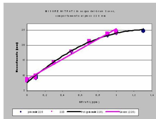
Fig.2 Nitrate UV absorption vs. concentration
