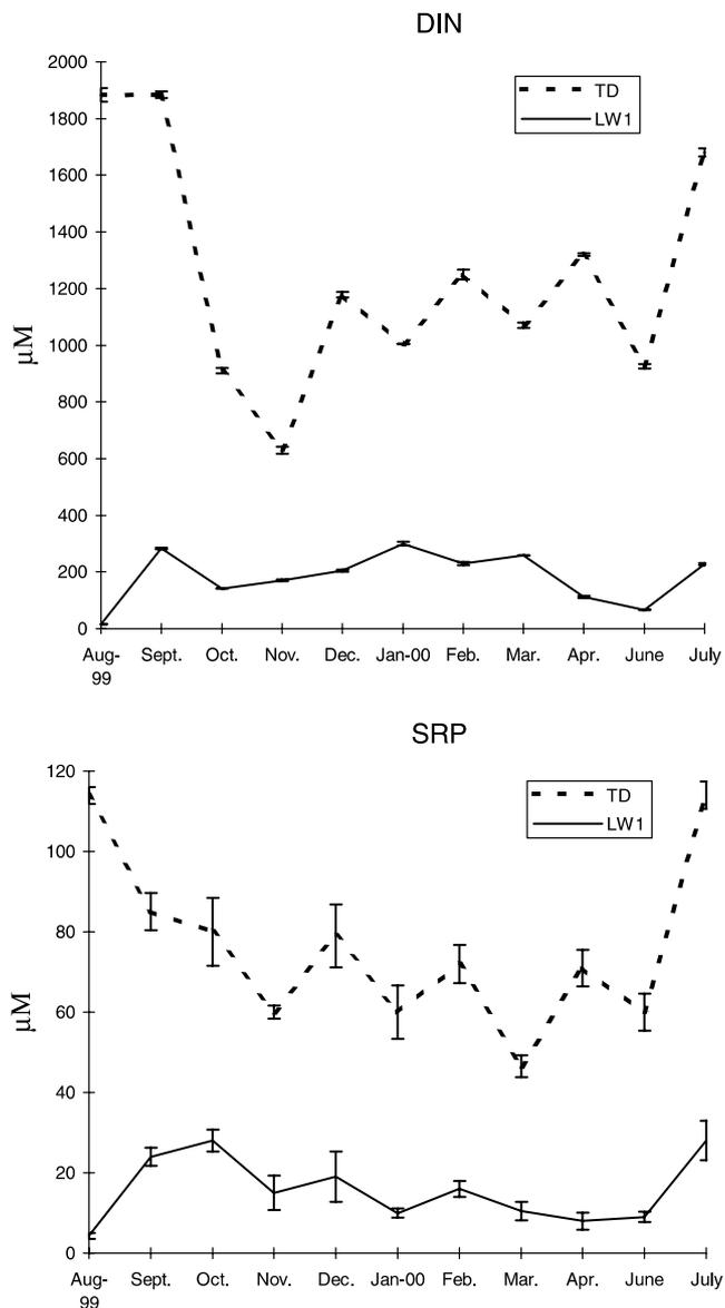
Fig. 4. Means ( $\pm$ SD) of dissolved inorganic nitrogen (DIN) and soluble reactive phosphorus (SRP,  $P-PO_4^{3-}$ )  $\mu$ M, for urban wastewater treatment effluent (TD) and for effluent from the relative phytotreatment area (LW1), for 1999–2000.
