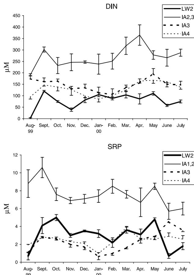
Fig. 5. Means ( $\pm$ SD) of dissolved inorganic nitrogen (DIN) and soluble reactive phosphorus (SRP,  $P-PO_4^{3-}$ )  $\mu$ M, for the effluent from the four intensive aquaculture plants, IA1, IA2, IA3, IA4, and for the effluent from the phytotreatment area of the first two (LW2).
