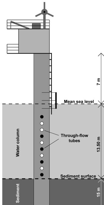
Figure 2. Sketch of the observatory (modified after [3]). Through-flow tubes marked in white are equipped with sensors, whereas tubes in black are closed.
