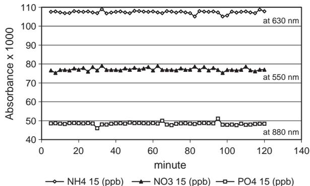
Fig. 5. Instrument drift—a standard solution (15 ppb) for ammonia, nitrate and orthophosphate in seawater was analyzed, every 150 s.
