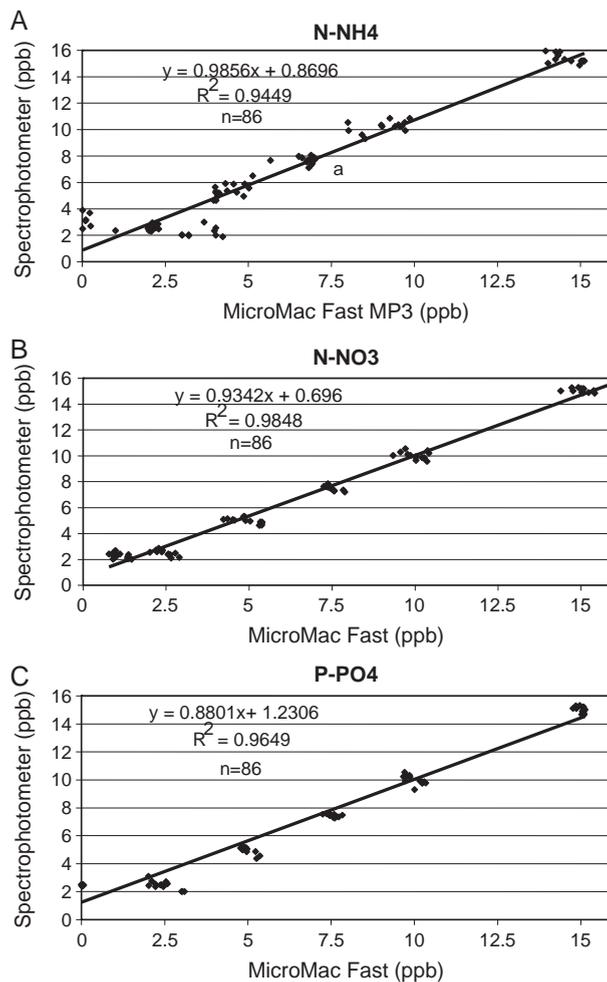
Fig. 4. Linear regression analysis relationship between automated and manual determinations of ammonia (A), nitrate (B) and orthophosphate (C).
