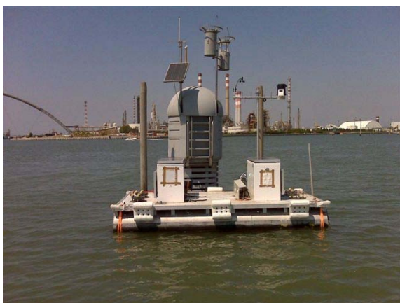
Fig. 1 WARMER water quality monitoring platform moored nearby VE-5 station
