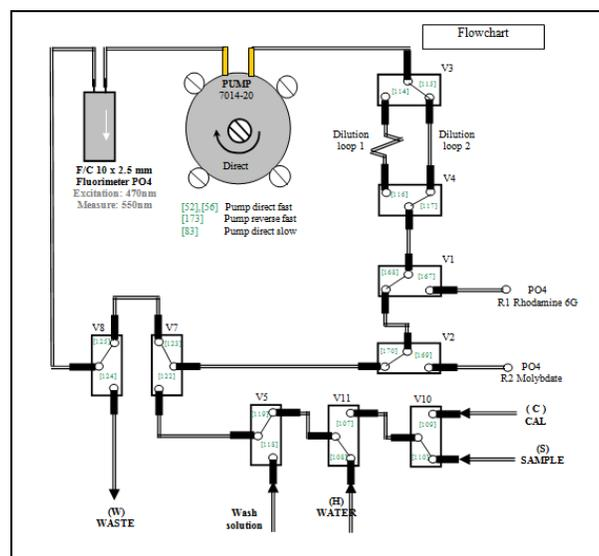
Fig. 4. The  $\mu$ LFA hydraulic circuit for fluorimetric phosphate analysis.
