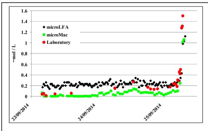
Fig. 9. Ferrybox PO<sub>4</sub> measurements performed with μLFA module (black diamonds), Micromac-1000 (green squares) and with a CFA instrument in laboratory (red dots).
