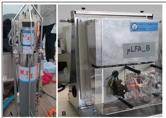
Fig. 3. The WIZ in-situ probe (A) and the  $\mu$ LFA module (B).
