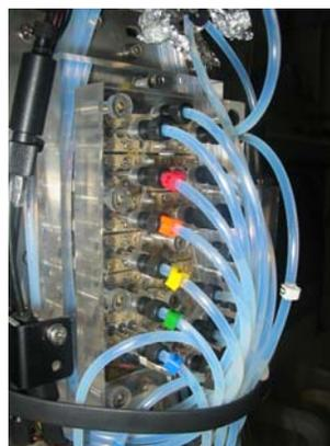
**Fig. 2 The  $\mu$ LFA hydraulic manifold**
