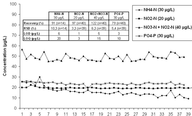
Fig.4 DPA repeatability and accuracy test results
