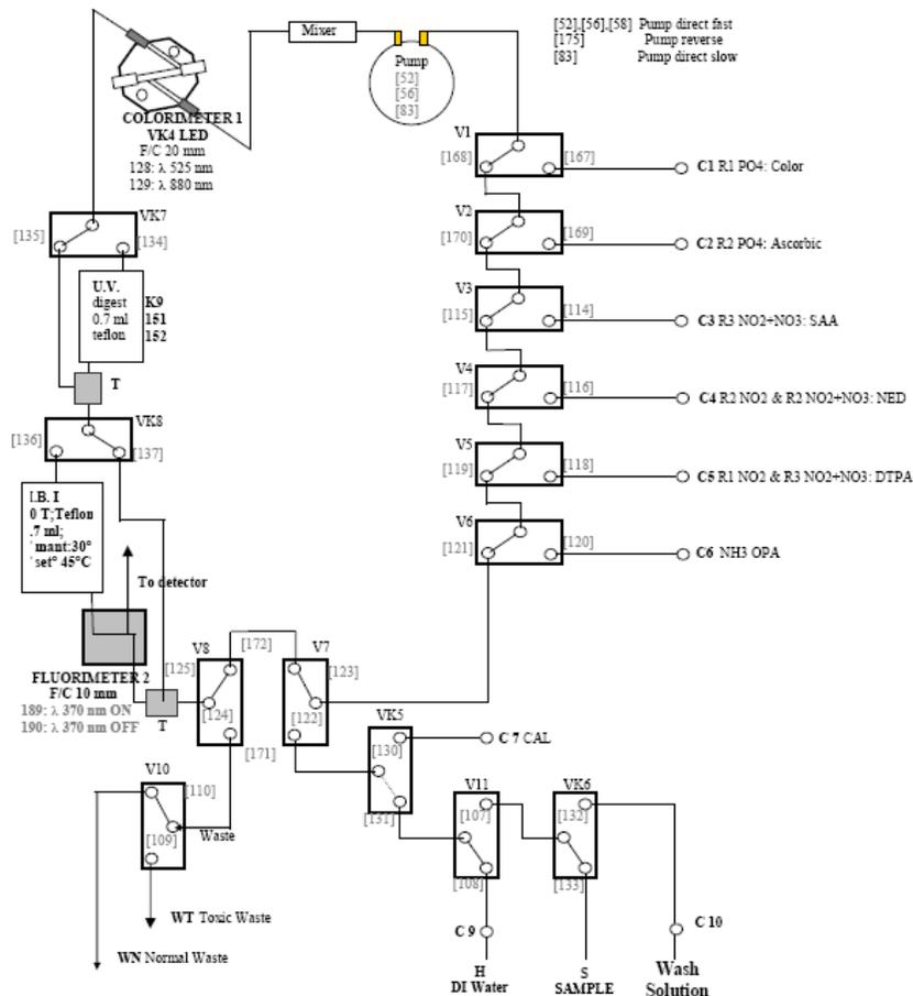
**Fig. 3  $\mu$ LFR schematic hydraulic diagram**
