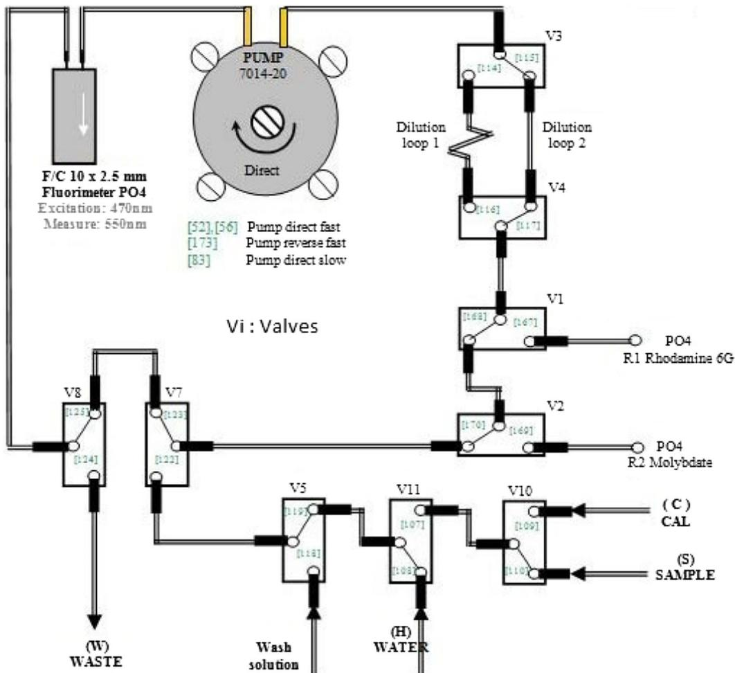
Fig. 3 μLFA hydraulic circuit for direct fluorimetric phosphate analysis (SYSTEA 2016)
