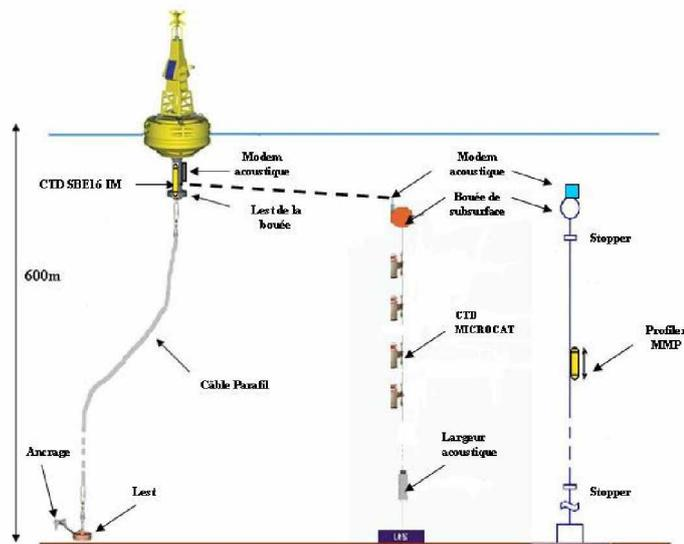
Fig. 6 MOLA buoy final design
