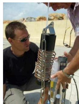
**Fig. 9 On line filter with copper wire**
