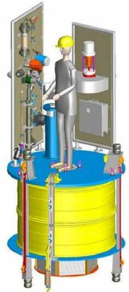
Fig. 2 MAREL CARNOT autonomous station drawing with NPA implemented (blue cylinder)
